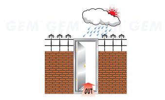
This series of Waterproof Magnetic Lock is made with epoxy potting compound and is protected by this compound. Also, GEM Waterproof Series Magnetic Locks have been proved to have withstood a water resistance as established in accordance with the test procedures of IPX7, IPX8 through a trusted third party. Therefore users need not worry that the lock will be rusted or sparked, if the lock is using in outdoor applications and installing in confined space where any inflammable gas.
